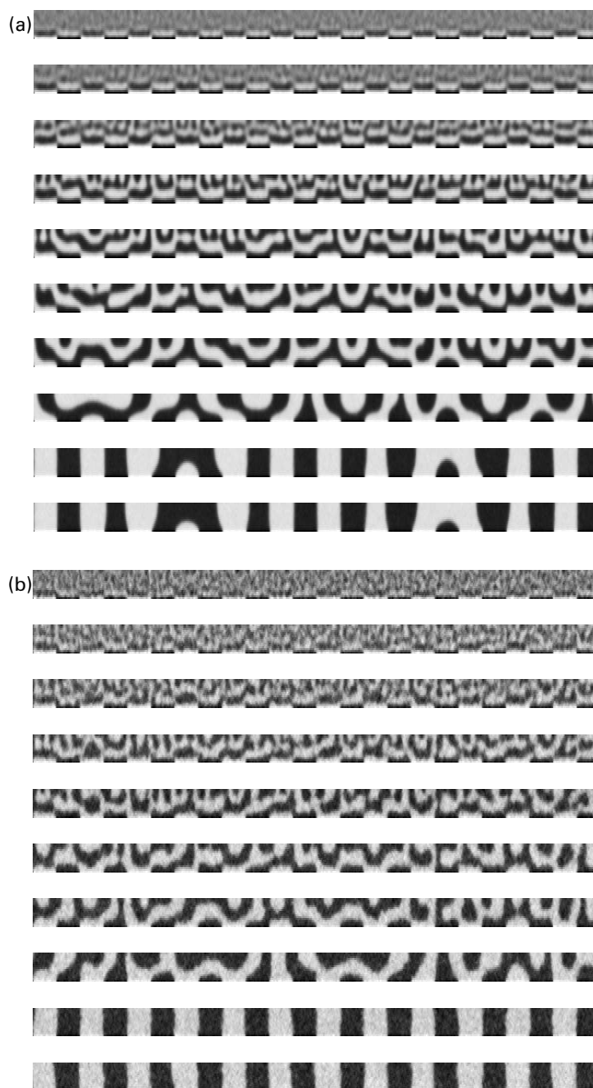
Fig. 7. Snapshots during the evolution of a thin film cast on a chemically patterned substrate under a temperature quench to two different final temperatures. In each case, the time sequence from top to bottom is t = 3, 6, 12, 24, 48, 96, 192, 768, 10,800, 24,000 . The width of the surface pattern ( \omega = 24 ) and the surface interaction strength ( \sigma = 1 ) are the same in each case. In (a) the noise strength \varepsilon = 0.01 while in (b) it is given by \varepsilon = 0.6 .
